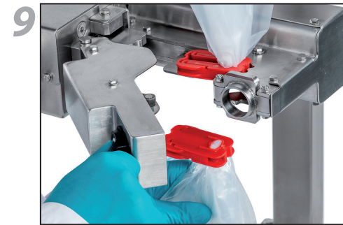
Both parts are tightly closed and can be removed after opening the tool
