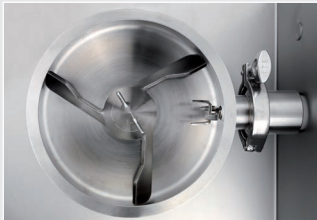
Standard mixer granulator: elevated blade tips
