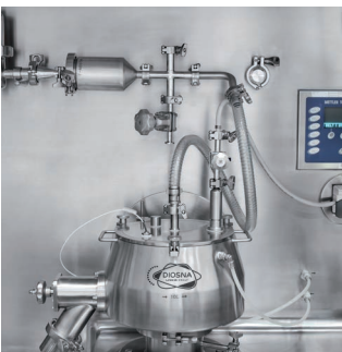
Detail Isolator Installation with vacuum drying.
