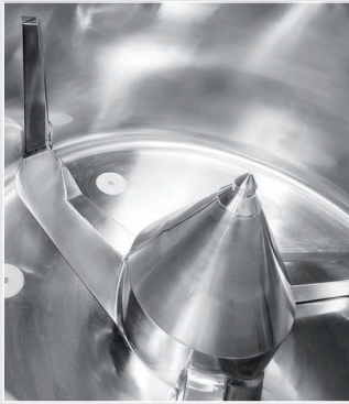
Vacuum drying: Tool blade with stripper.
