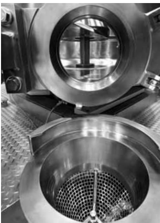
Opened discharge valve and Tool-lift of the mixer-granulator.
