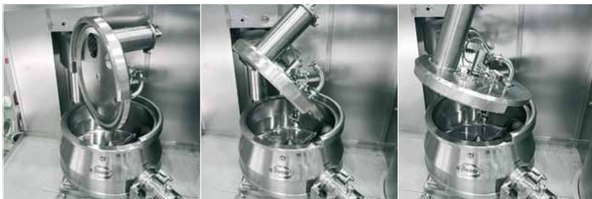
12 bar pressure shock resistant mixer-granulator with innovative automated lid actuation.
