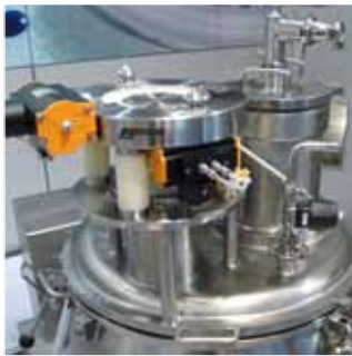
Containment design of mixer lid with split butterfly valve
