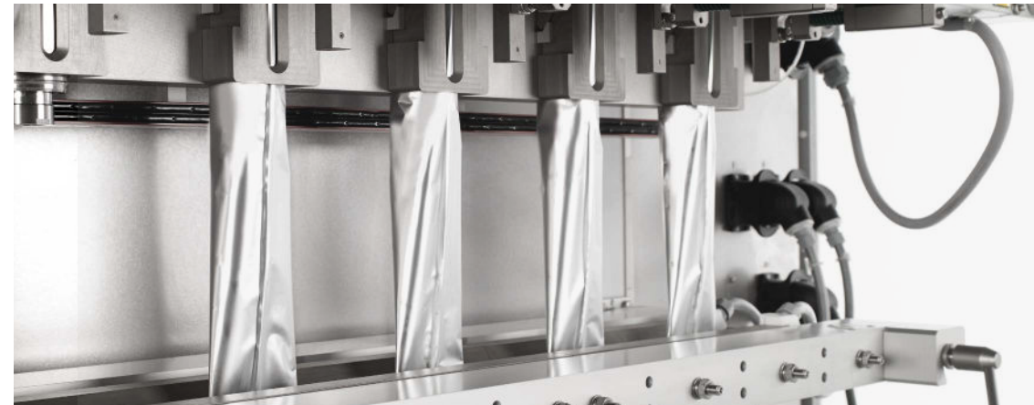
Detail of a Stick Pack machine former.
